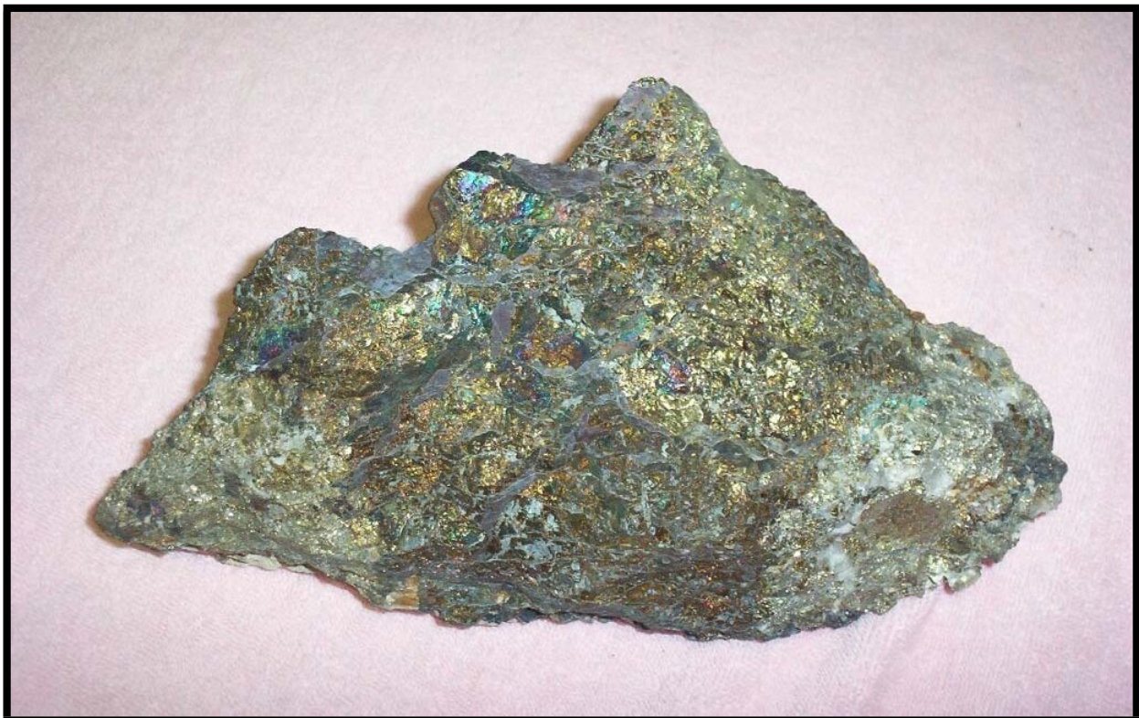
Figure 3. Photograph of Victoria ore, consisting primarily of bornite and chalcopyrite.
